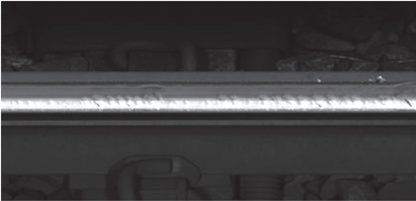
Fig. 3.17 Picture of head checks taken with new image system
