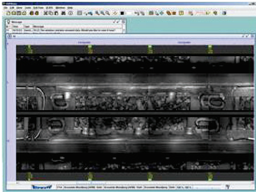
Fig. 3.9 Former image system for rail head surface
