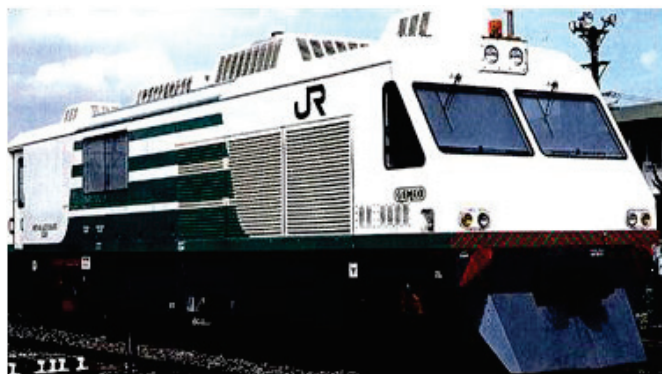
Fig. 1.17 Rail flow detection vehicle (RFD)
