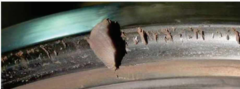
Fig. 4.41 Situation of rail disk head after 10.6 million rotations
