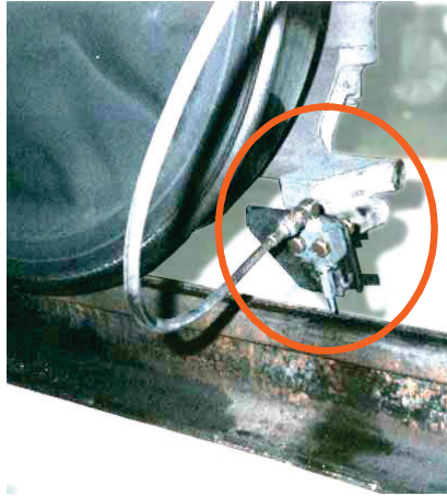
Fig. 2.11 On-board lubricant system for rail
