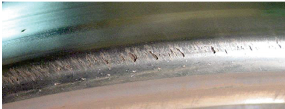
Fig. 4.40 Situation of rail disk head after 7.8 million rotations
