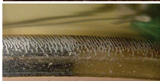
Fig. 5.4 Situation of rail disk head at 10.5 million rotations
