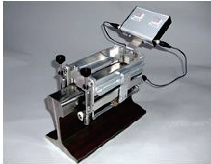
Fig. 3.21 Ultrasonic flow detector detecting vertical crack from upper fishing surface of rail head
