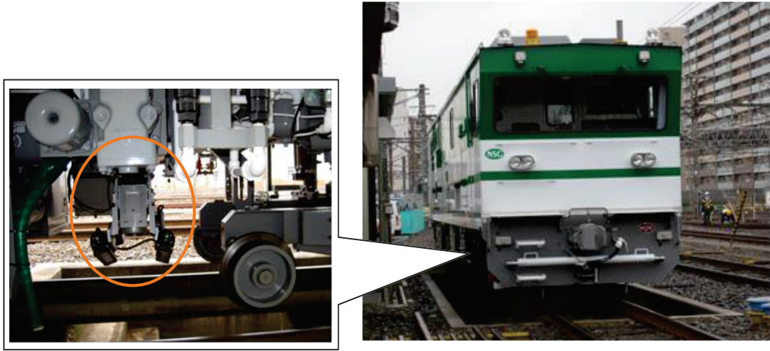
Fig. 3.16 Image system installed on the newest rail flow detecting car
