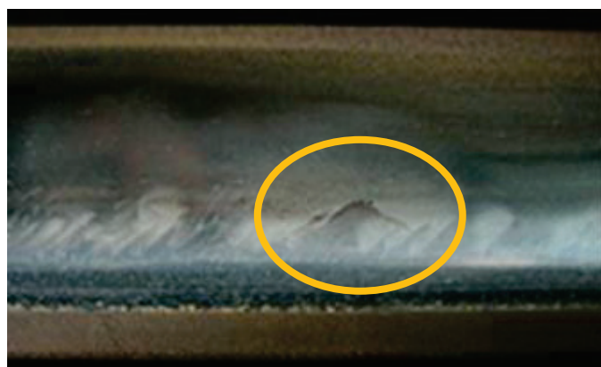
Fig. 1.12 Gage corner cracking
