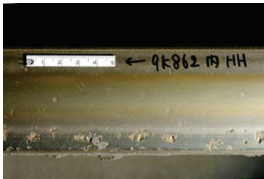
Fig. 2.13 Pitting at curved track lubricated by on-board system
