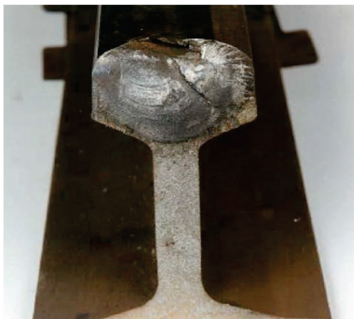
Fig. 1.36 Cross section of rail break at the accident point [22]
