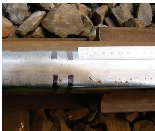
Fig. 2.7 Head checks at a research line in 2004
