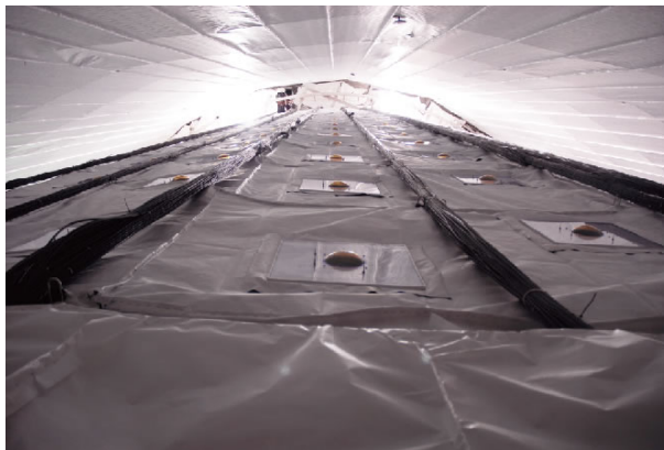
Figure 3.4: A photo from the bottom of the outer region. The PMTs with 20 cm diameter are mounted with wavelength shifting plates on the wall on the side of the ID, and the OD is surrounded by a white Tyvek sheet [25].
