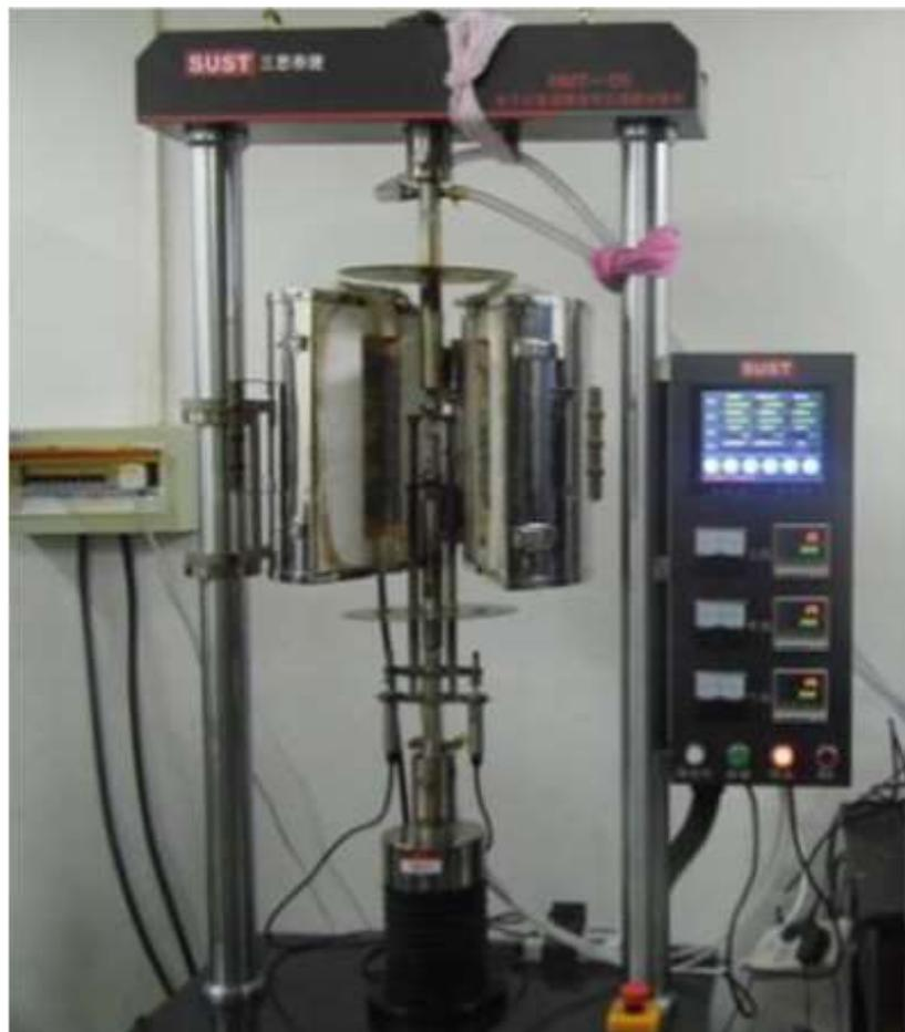
Figure 2-17 Creep test set-up for Q460 steel (Wang W., 2017)
