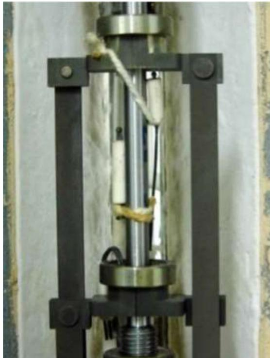
Figure 2-19 Thermocouples set-up (instrumentations on test Q460 specimen) (Wang W., 2017)
