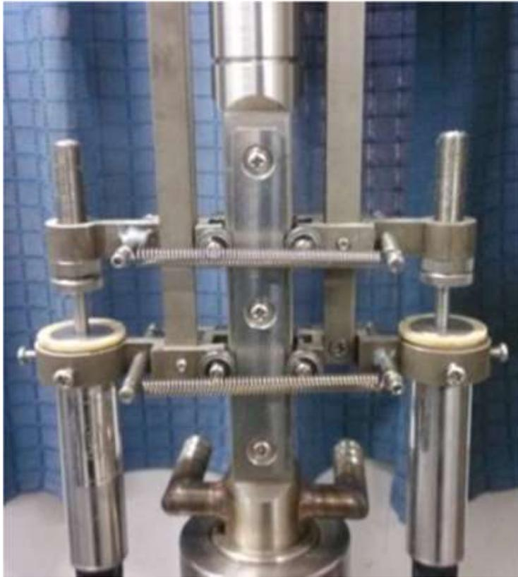
Figure 2-18 LVDTs systems (instrumentations on test Q460 specimen) (Wang W., 2017)
