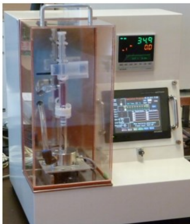
Fig. 2-3 Falling needle rheometer [113]
