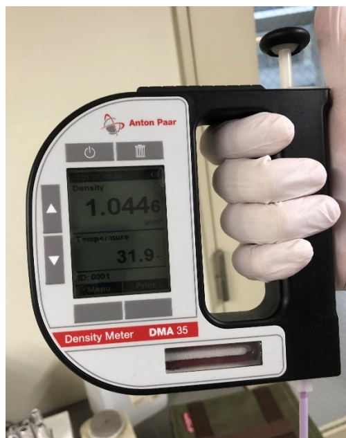
Fig. 2-5 Portable densimeter (DMA35)
