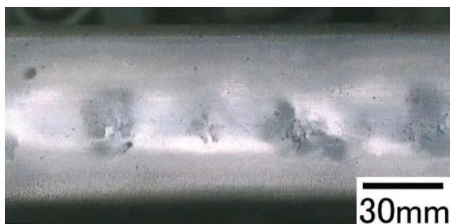
Fig.3.1 Typical damage observed on the running surface of the rail used in this study. The upper side is the field corner side and the lower side is the gauge corner side.
