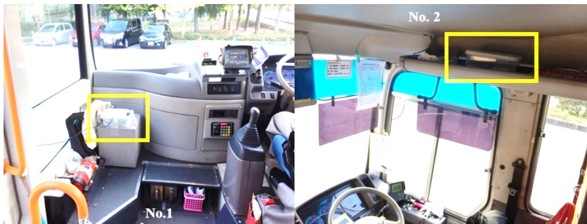
Figure 4. Wi-Fi scanners installed on buses No. 1 and No. 2
