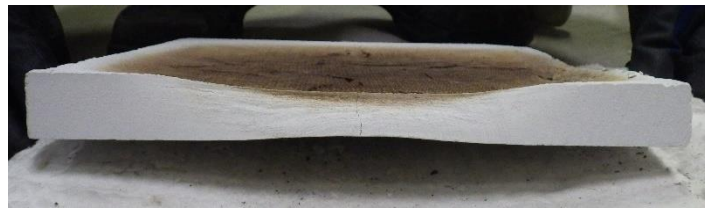
Fig. 2.3.3 加熱後の断面状況(CSB d_i = 25\text{mm} , d_s = 6\text{mm} , \alpha = 650 )
