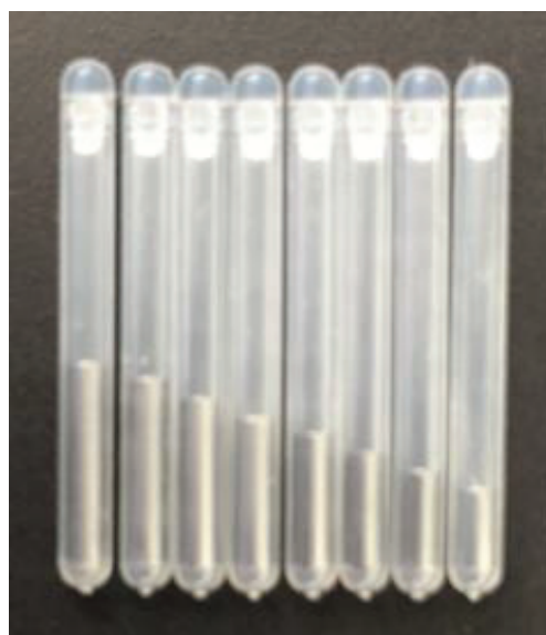
Fig. A-2 Cylindrical needles used in rheometry with the FNR
