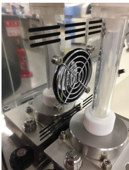
Fig. A-3 Constant temperature air circulation system
