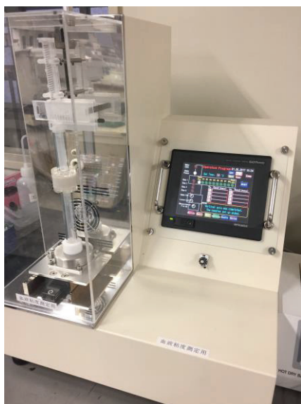
Fig. A-1 Falling needle rheometer (FNR)
