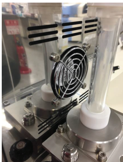
Fig. A-3 Constant temperature air circulation system
