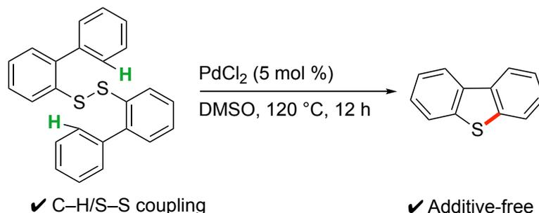
**Scheme 4-1.** C–S bond formation with PdCl<sub>2</sub>/DMSO catalytic system
