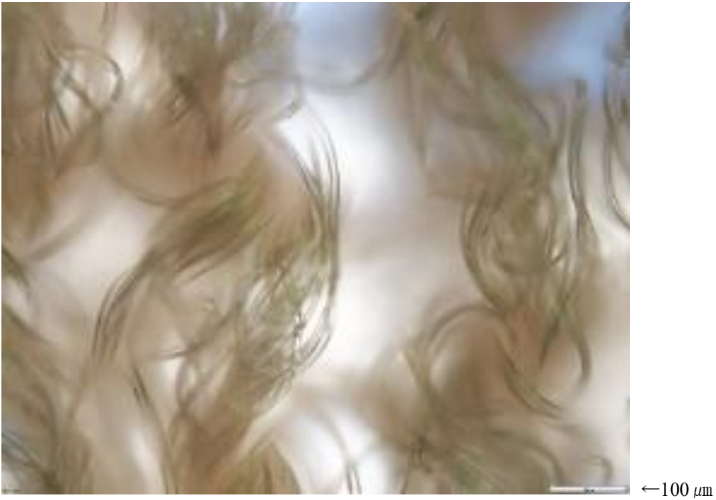
Fig. 18(a) Surface microphotographs of Naboal. OLYMPUS Microscope BX53 at 100 (10 x 10) times. The white bar on the bottom right indicates 100 \mu\text{m} .
