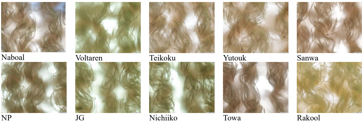
Fig. 18 (b) Surface microphotographs of various tapes. OLYMPUS Microscope BX53 at 100 (10 x 10) times. The white bar on the bottom right indicates 100 \mu\text{m} .
