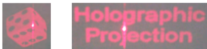
Fig. 6.1 Laser patterns by reflection of the red diode laser beam on the LCOS-SLM.
