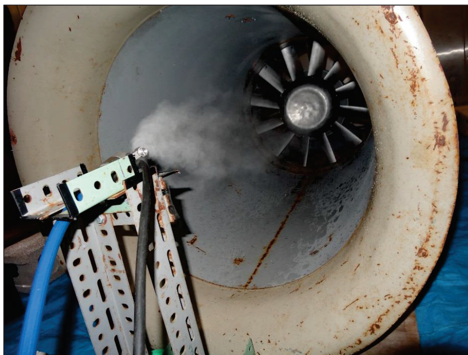
Fig. 4-1 Icing Test Facility for Axial Fan
