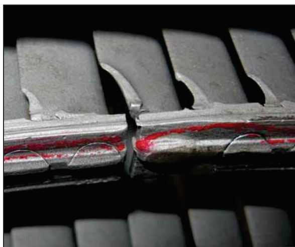
Fig. 1-1 Erosion of Compressor (1)
