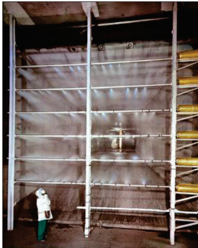
Fig. 1-16 Spray Bar System for IRT at NASA GRC (23)
