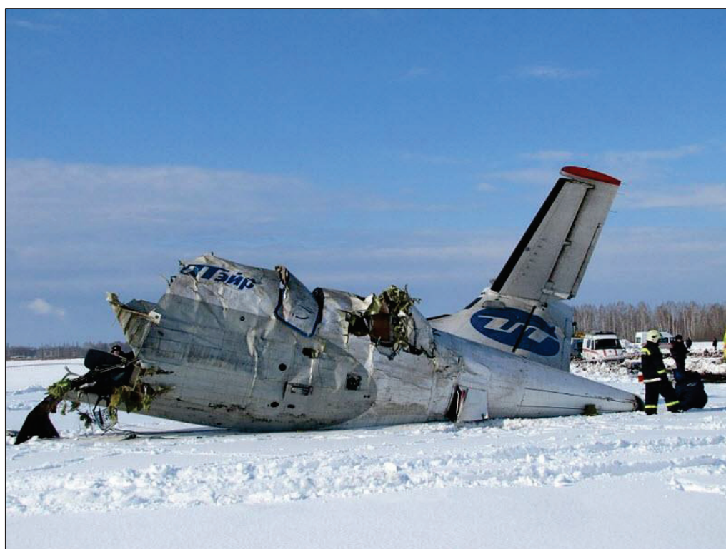
Fig. 1-14 Icing Accident of UT Air 120 (20)
